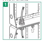
Add-on possibility Enclosures can be horizontally or vertically associated keeping the IP65 and allowing
